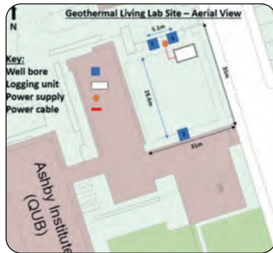
Figure 3 QUB Geothermal Living Lab
