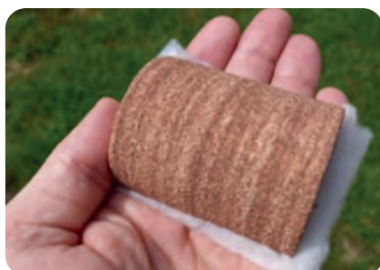
Figure 1 – Sherwood Sandstone core sample
