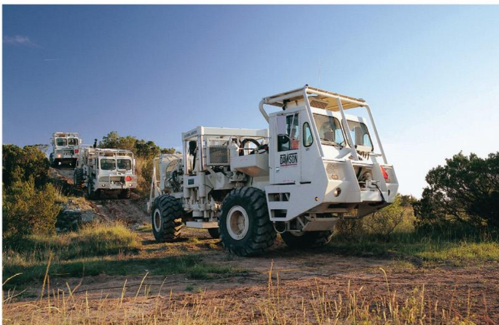
Trucks thumping on the ground to generate the signal needed for making a seismic-reflection profile.
