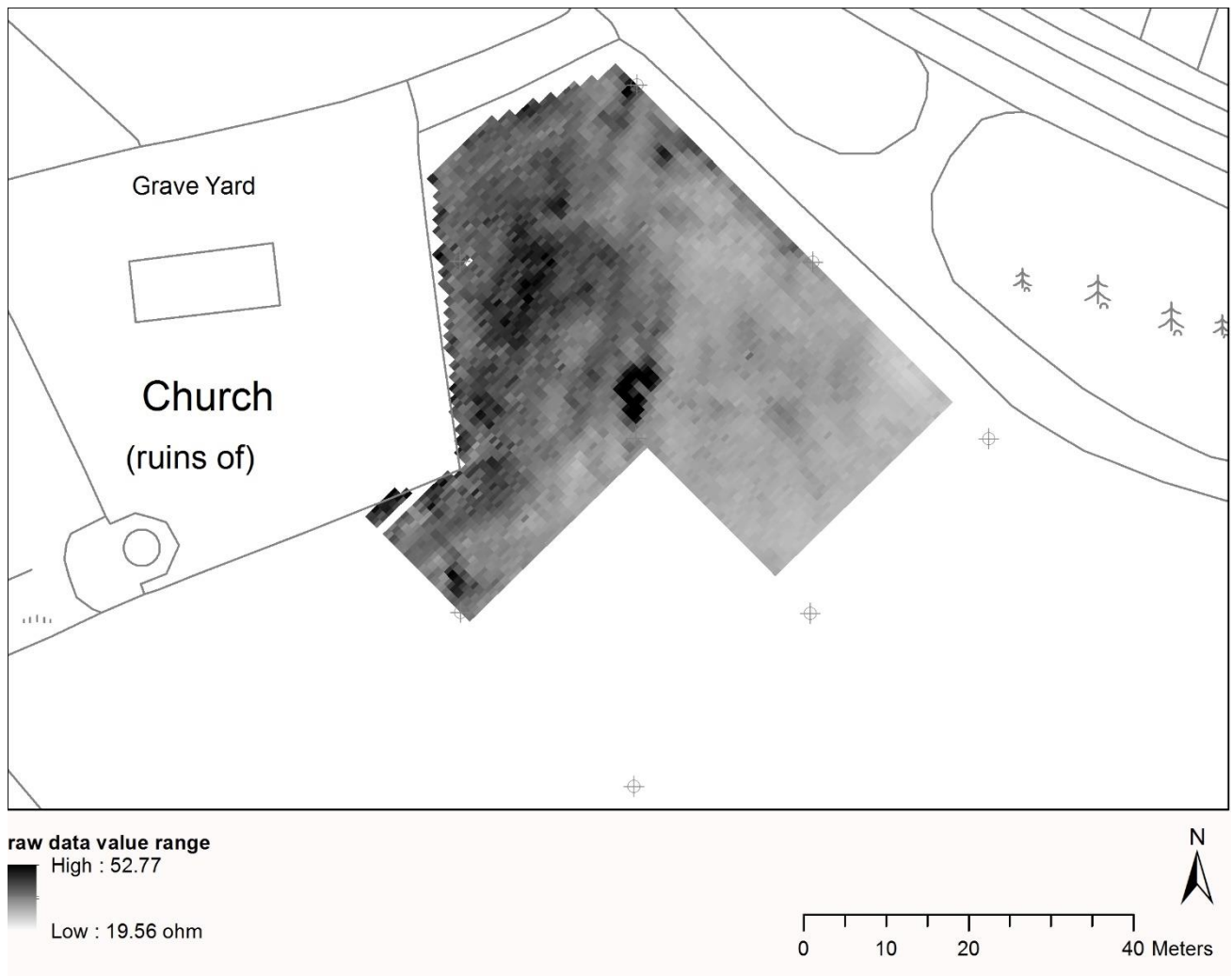
Figure 6 Greyscale plot of raw data clipped at 0/+100 Ohm and despiked.*
