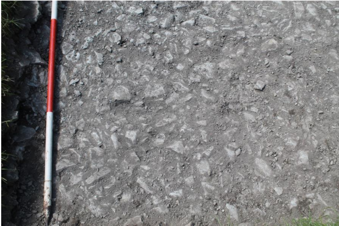
Plate 9 Surface of C507, illustrating the compacted nature of the stones and their worn/rounded surfaces.
