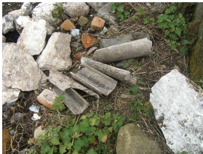
Examples of asbestos guttering. Centre for Archaeological Fieldwork
